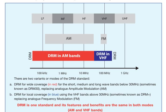
The way in which signals propagate at different frequencies is the same for DRM as for existing analogue transmissions. This will range from short wave frequencies that can cover very long distances over any type of terrain, to VHF that is meant for local coverage. This is illustrated below:
