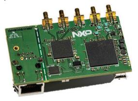
In addition, NXP demonstrated dual tuners and a costeffective single tuner on DRM platforms shown above. These tuners also support the traditional analogue frequencies.
