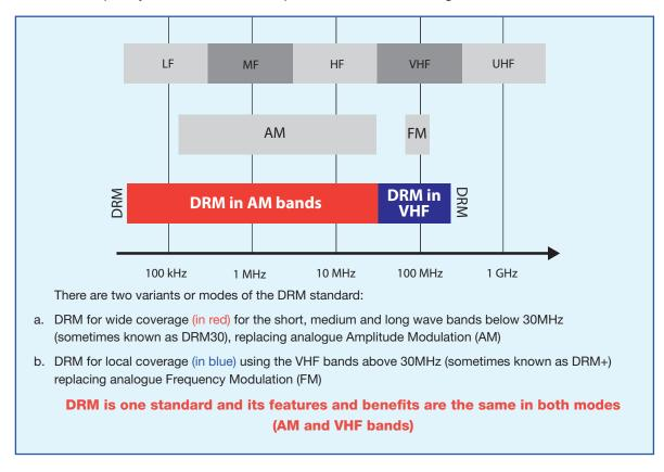
The way in which signals propagate at different frequencies is the same for DRM as for existing analogue transmissions. This will range from short wave frequencies that can cover very long distances over any type of terrain, to VHF that is meant for local coverage. This is illustrated below:
