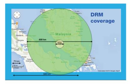
large area coverage, as illustrated here. The small circle shows the localised FM coverage, whereas the large circle illustrates the very large area by using DRM in medium wave.
