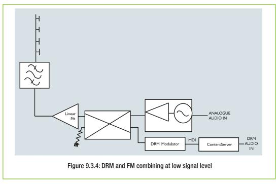
In this configuration the DRM signal and the FM signal are combined in front of the power amplifier. The coupling is done at low signal level and the energy losses on the dummy load resistor connected to the hybrid coupler is insignificant.
