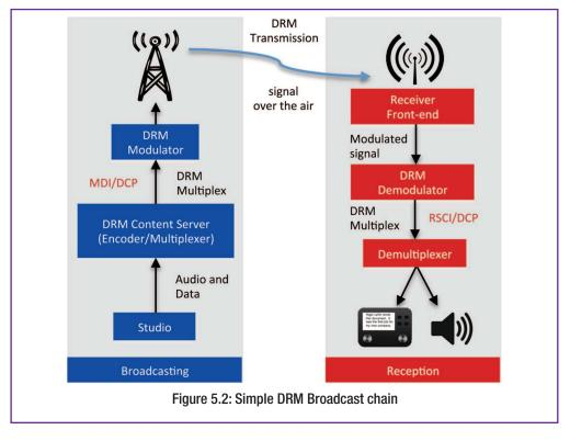
In the following sections we will examine the operation of the two main functional blocks shown above: the Content Server and the Modulator. In most (but not all) installations, these functional blocks correspond to commercially available products. They communicate via a Multiplex Distribution interface (MDI) over a Distribution and Communications protocol (DCP), both of which have been standardised [2], [3].
