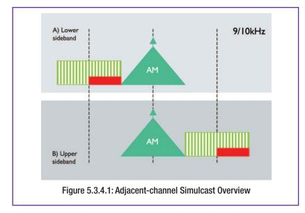
The conclusion is that a satisfactory compromise can be obtained when the level is around 14-16 dB below the adjacent analogue carrier level.
