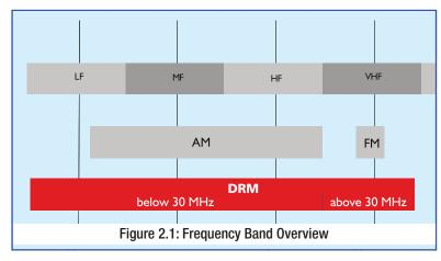
**DRM transmissions below 30 MHz:** 4 different robustness modes allow the DRM signal to be tailored for the AM broadcast bands with their very diverse propagation characteristics, enabling regional up to international service coverage.
