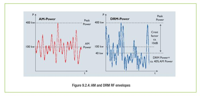
The DRM signal, as broadcast, closely resembles band-limited noise. This is an advantage when considering the protection ratio of analogue systems interfered with by DRM, but not when it comes to amplification. The statistical variation of envelope voltage theoretically follows a Raleigh distribution, but in practice the peak-to-mean ratio lies between 10 and 11dB<sup>15</sup>. Fortunately, current AM transmitter topologies can be adapted to amplify the DRM signal in an efficient manner.
