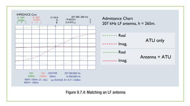
Where system bandwidth (in terms of the VSWR characteristic — which can also usually be obtained from the Network Analyser), is less than optimum, the first line of approach is to consider the transmitter and antenna system response as a whole. The overall response is then measured and used to determine the pre-correction required at the DRM Modulator and so compensate for the restricted antenna bandwidth
