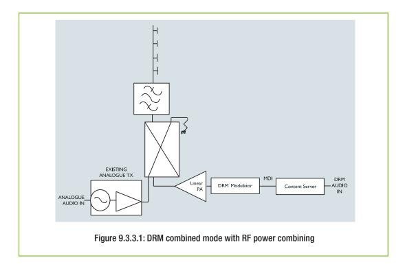
Transmission power is lost in the dummy load connected to the necessary hybrid coupler, but the advantage is that the analogue and digital chains are fully independent in operation.
