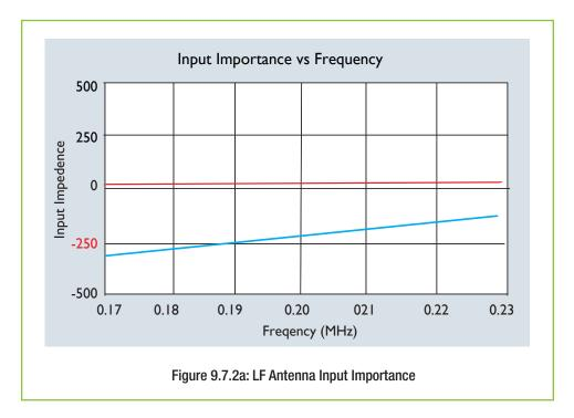
The **red** curve represents the resistive component and the **blue**, the reactive component. As can be seen the antenna is predominantly capacitive with a very small resistive component, typically this is of the order of 5 - 10 Ohms.
