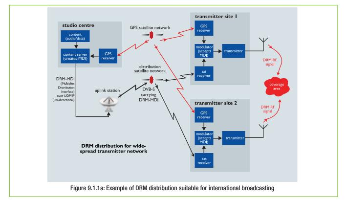
The data is sent asynchronously in packets. Therefore a large variety of basic transport mechanisms may be used, such as UDP/IP, serial lines, Satellite, WAN, LAN, and ISDN. As the multiplex is based upon either a 100ms or 400ms DRM frame, and the transmission of data is effected asynchronously, both the DRM multiplexer and modulator must possess their own source of time synchronization (GPS or Network Time Protocol, **NTP**), to ensure the long-term stability of this framing.
