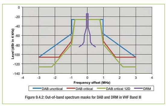
Table 9.4.2: Out-of-band spectrum masks for DAB and DRM in VHF Band III
