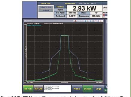
Figure 9.3.2b: DRM transmitter; measured output spectrum for a 3 kW transmitter
