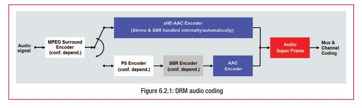
Both encoders can operate over a range of bit rates, and consequently support a range of programme content. For DRM configurations that provide higher content capacity, 5.1 surround sound broadcasts are supported by the MPEG Surround technology, which is backward compatible with mono and stereo receivers.
