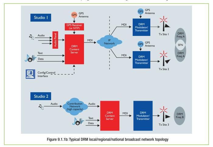
For broadcasters wishing to retain their present audio programme distribution network and not intending to use any of DRM's advanced value-added services, placement of the Content Server at the transmitter site is acceptable. However, to retain the superior audio quality of the DRM system requires that the programme be distributed at the highest possible bit rate in order to minimize tandem-coding artefacts.
